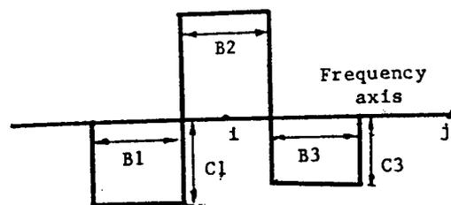
Figure 1. Spectral lateral inhibition filter.
