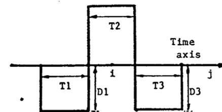
Figure 2. Time-domain lateral inhibition law.
