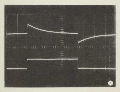
Fig. 1. A. Response of the glottograph to a rectangularly shaped resistance increase. The direct output with a long time constant preserves the waveform.
