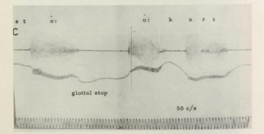
3. C. Glottal stop marking a word boundary shows up as an extreme low resistance in the electrical glottogram. The Mingograph channel displaying the output of the electrical glottograph lags the speech oscillogram trace by 15 msec as indicated by the vertical line. This instrumental factor affects (A), (B), and (C).
