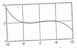
Fig. 2. Departure from linearity of the semitone scale obtained by an exponential approximation with the time constant equal to the period of the center frequency. Horizontal axis: log frequency in semiones re center frequency; vertical axis: deviation of the actual scale from a linear one, in semitones. This may be taken into account when calibrating the instrument or, in one-octave range, it may be neglected being less than  $\pm 5$  C.
