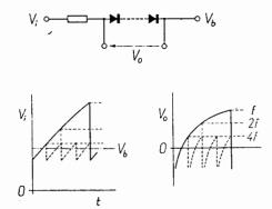
Fig. 1. Simple quasilogarithmic network transforms the initial, approximately linear, portion of an exponential function into logarithmic function within the range from f to 4f.  $V_i$  — input voltage from an instantaneous frequency meter based on (3),  $V_0$  -- logarithmic output fed to a differential amplifier with high input impedance,  $V_b$  — fixed bias voltage. Instead of one, several diodes are connected in series to increase  $V_0$ .
