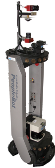
(d) The mobile robot used for acquiring the data. The cameras and the laser scanner can be seen on the top and bottom platforms, respectively.
