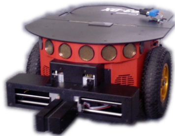
(b) P3-DX by MobileRobots Inc.: a wheeled mobile robot.
