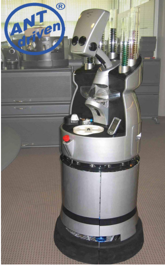
(a) The Nesbot robot by BlueBotics: a mobile service robot with limited user interaction capabilities.
