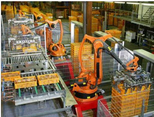
Figure 2.1: Factory Automation with industrial robots for palletizing food products like bread and toast at a bakery in Germany.
