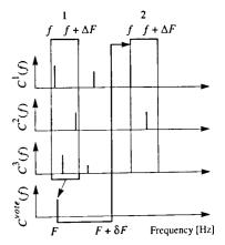
Figure 1: Example of two iterations of the combination mechanism for formant frequency estimation.
