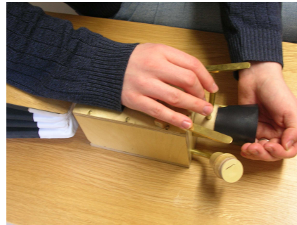
Figure 1: Photograph of the inner life of the speaking machine while being played: palm of the hand on the right forming vowel resonances in front of a rubber funnel (vocal tract); the hand on the wooden windchest (thorax) regulating nasal cavity resonances; (invisible) elbow providing pressure on the bellows (lungs). The reed pipe is located within the "nose".
