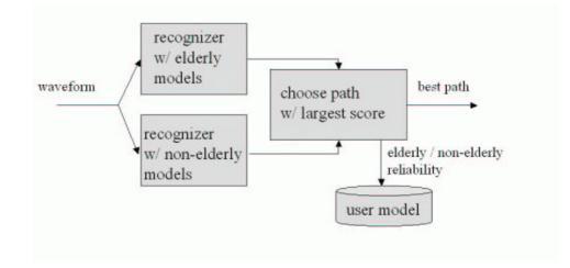
Figure 5. Diagram of a parallel age dependent recognition system
