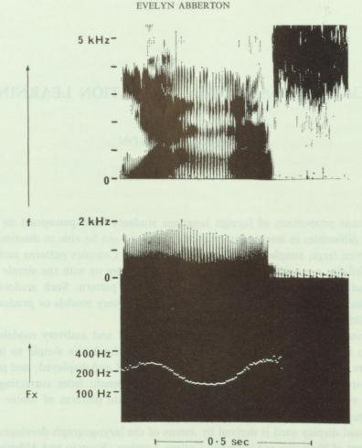
Fig. 1. The top photograph is a spectrogram of the word Yes spoken with a falling-rising intonation pattern. The centre photograph shows a spectrogram of the corresponding Lx, giving no information about vocal tract resonances or friction; and the lower photograph shows a display of the fundamental frequency derived from the Lx of the middle photograph. This simply obtained display, of the type used in teaching, corresponds closely to our perception of intonation.
