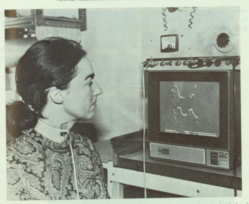
Fig. 2. A subject practising. She is wearing neck electrodes held in place by an elastic band. The combined laryngograph and fundamental frequency generator are to her left, and on the screen are two Fx traces for 'It's easy, isn't it?'
