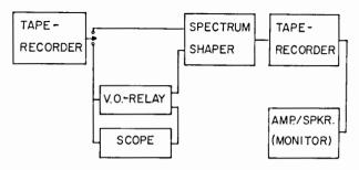
Fig. 1. Schematic of instrumentation used in modifying nasal speech of 6 cleft-palate speakers.
